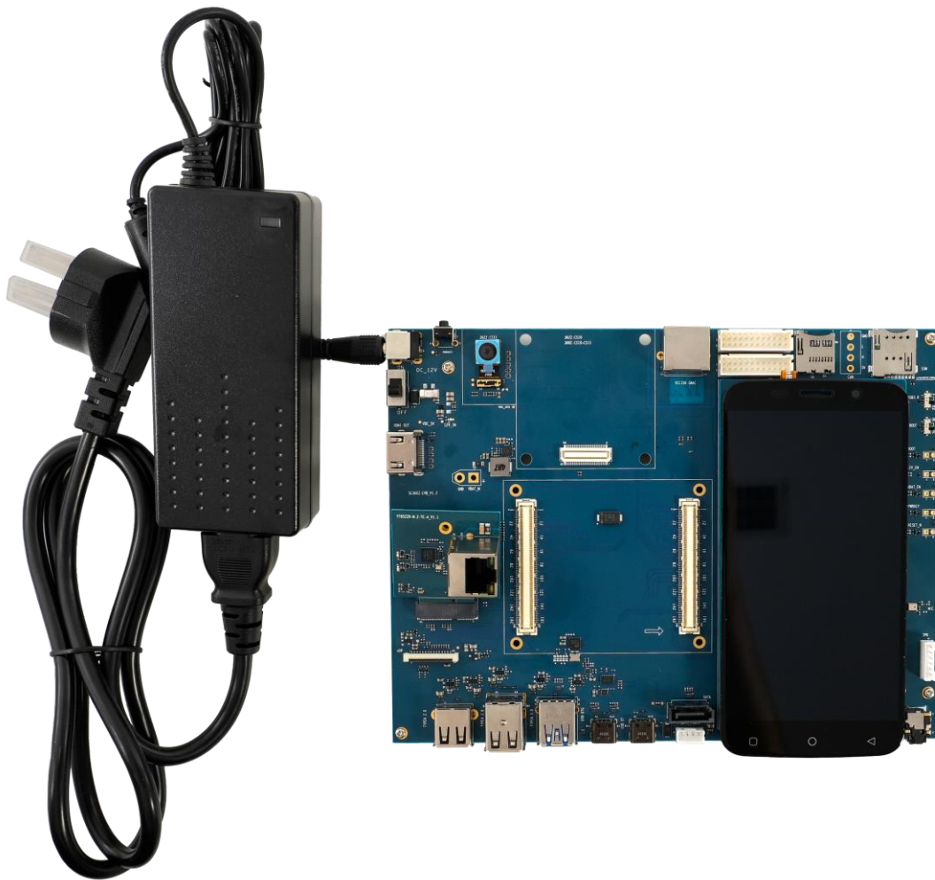
Figure 5: EVB and Accessories Assembly
